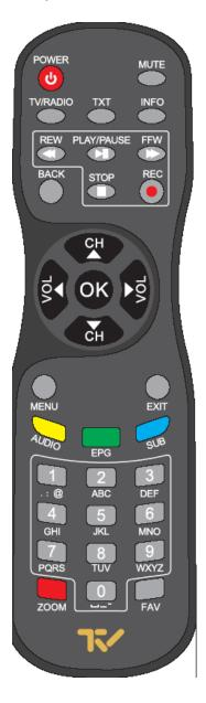
Power: The power key turns the STB on and off.
